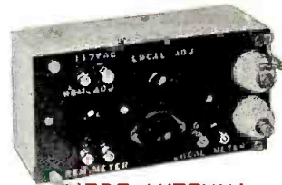
DIODE ANTENNA CURRENT METERING
